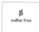
Figure 1 - Example of marking of 10 mg/kg sulfur
