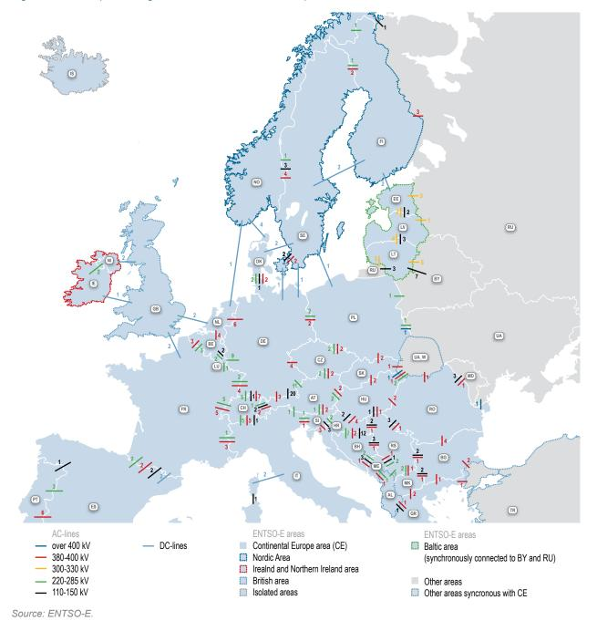
Figure 56: Simplified diagram of interconnectors in Europe
