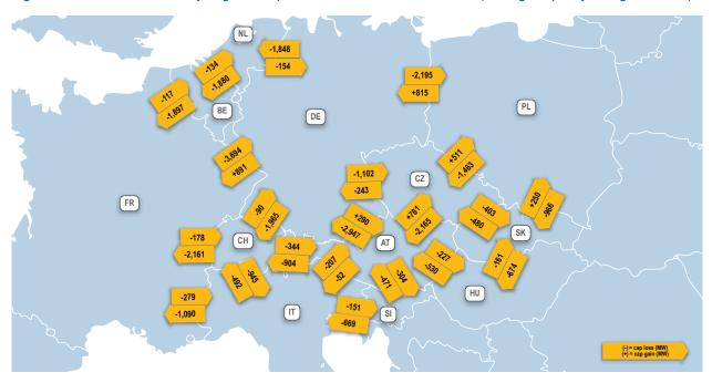
Figure 16: UFs with a mainly negative impact on cross-zonal trade – 2015 (average capacity loss/gain in MW)
