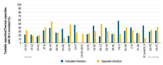
Table 15: Ratio between available NTC and aggregated thermal capacity of interconnectors without and with N-1 assessment – 2015 (%)
