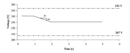
Figure 3a - A Rapid voltage change: Gradual change indicating the voltage change per time (dv/dt). The maximum change equals 10 V and the steady-state change equals 10 V.
