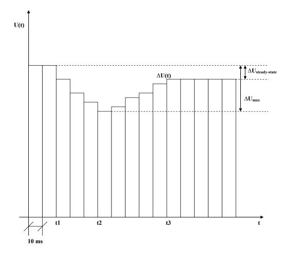
Figure 7 - A representative voltage change characteristic, with statement of rapid voltage changes.  $U(t) = a \text{ voltage change characteristic, } \Delta Umax = maximum \text{ voltage change and}$  $\Delta Usteadystate = steady-state \text{ voltage change.}$
