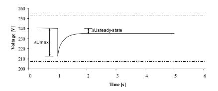
Figure 3c - A Rapid voltage change: Exponential change, typical due to the start-up of an induction motor. The maximum change equals 27 V and the steady-state change equals 5 V.
