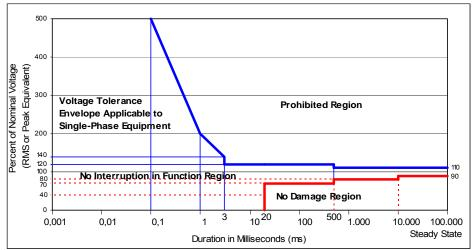
Figure 1 - The Information Technology Industry Council (ITIC) curve.
