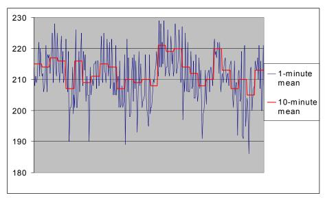
Figure 2 - The voltage RMS value measured as a ten-minute and one-minute average simultaneously in the same point of connection. The ten-minute and one-minute average is below 207 V 3,5 % and 28 % of the time respectively. Source: SINTEF Energy Research (Norway).
