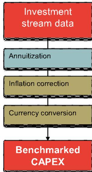
**Figure 4-3 Steps in deriving benchmarked CAPEX.**
