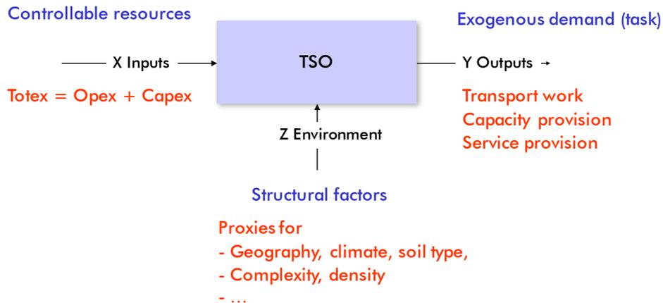
**Figure 4-5 Conceptual benchmarking model**
