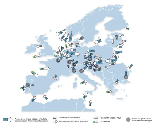
Figure 76: EU gas cross-border IPs physical capacity utilisation – 2013 (%)
