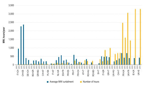
Figure 64: Average curtailed capacities and number of curtailed hours per border – 2012 and 2013 (MW and hours/year)
