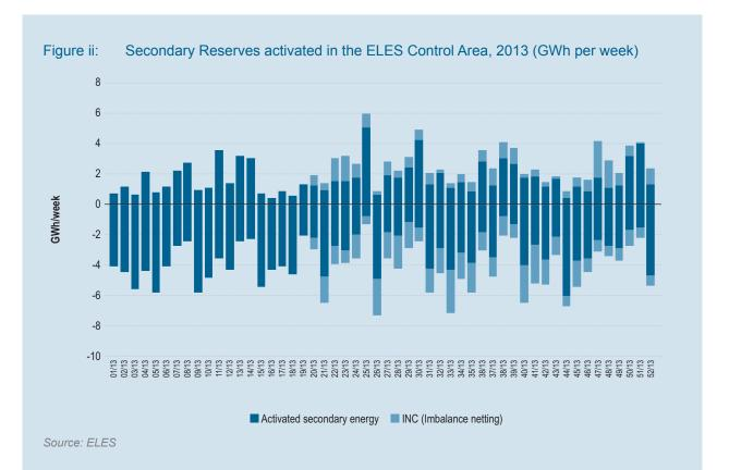
In April 2014, APG also joined the "International Grid Control Cooperation" (IGCC) project involving the cooperation of TSOs within, and on some borders of, Germany. Since then, imbalance netting in APG area has been performed in two steps. First, the imbalance netting is applied with ELES and second, the remaining imbalance of APG control area is netted within the IGCC project.
