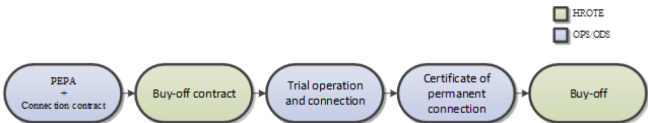
Figure 4.6.3 Simplified order of issuing acts in the preparation of the construction of integrated solar power plants
