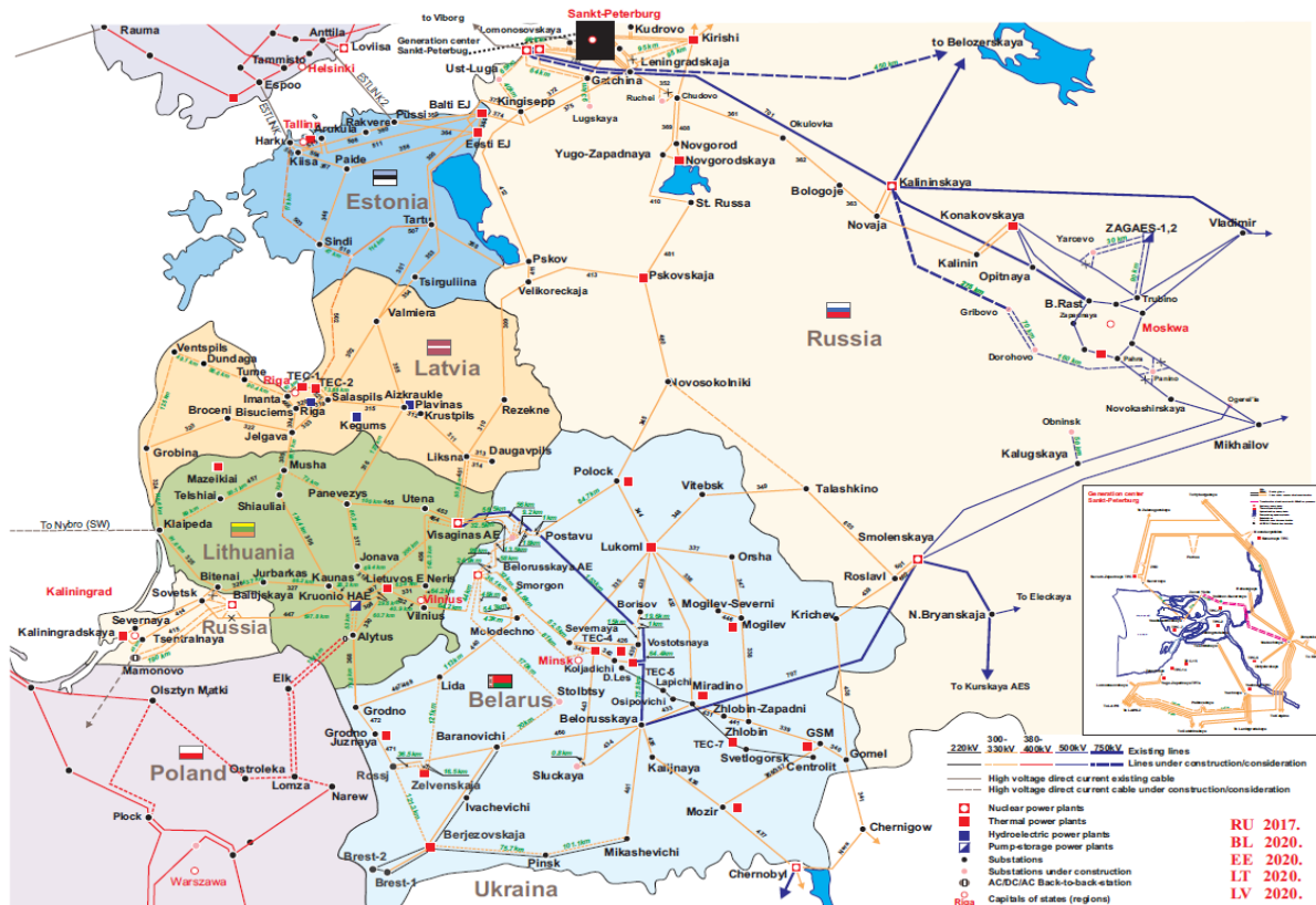
Figure 3. Map of electricity systems of Baltic countries and north-western part of Russia Source: Elering AS
