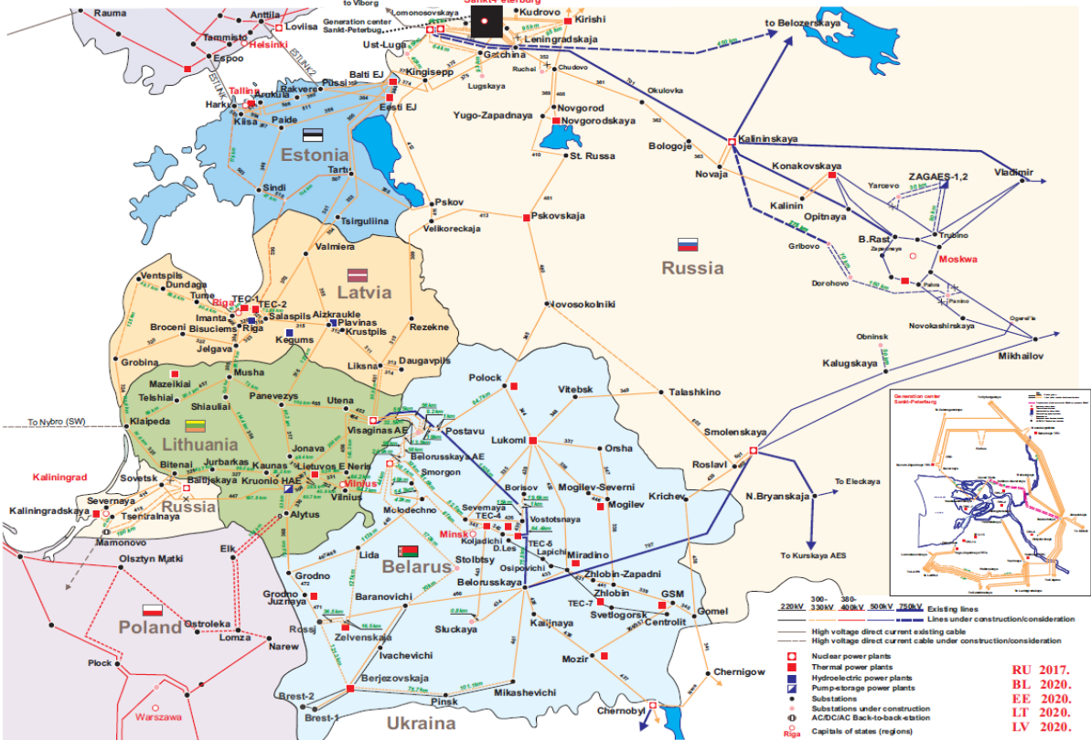
Figure 3. Map of electricity systems of Baltic countries and north-western part of Russia Source: Elering AS
