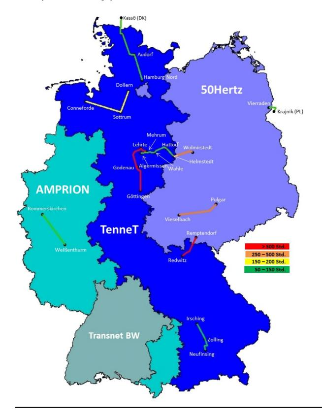
Figure 22: Electricity-related redispatch measures on the most strongly affected network elements in 2012 as notified by TSOs. Source: Own graph based on BNetzA GIS
