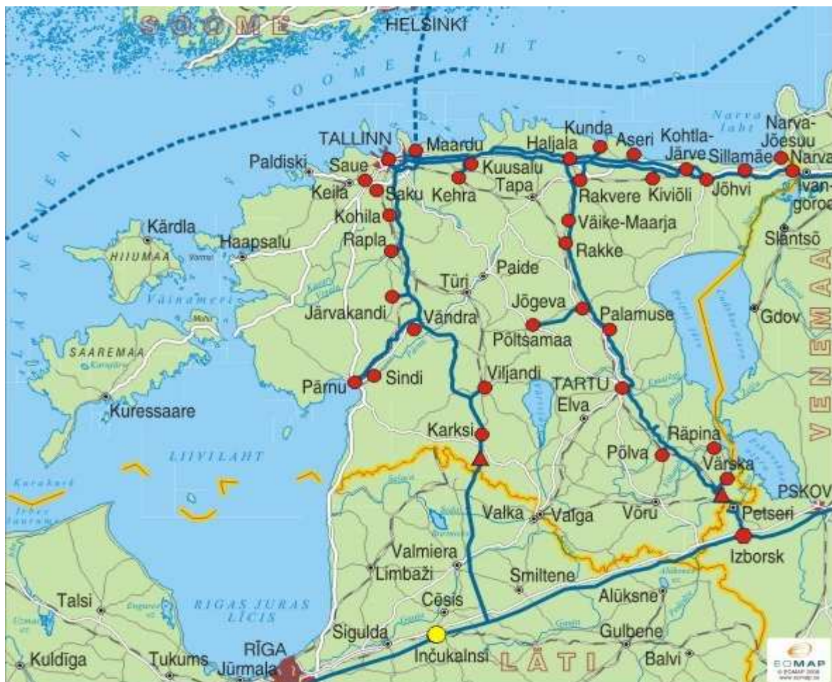
Drawing 4.1-1 Estonian natural gas transmission network (Source: AS EG Võrguteenus)
