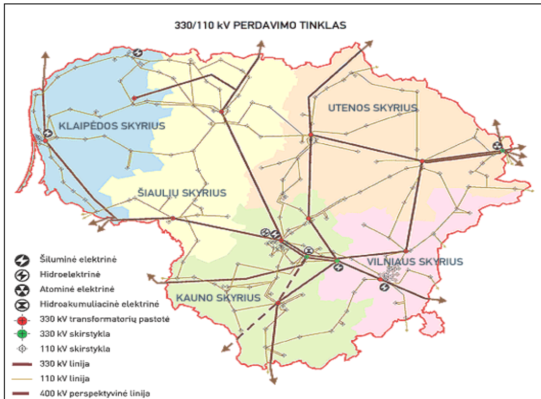
Figure 18. Lithuanian electricity transmission system
