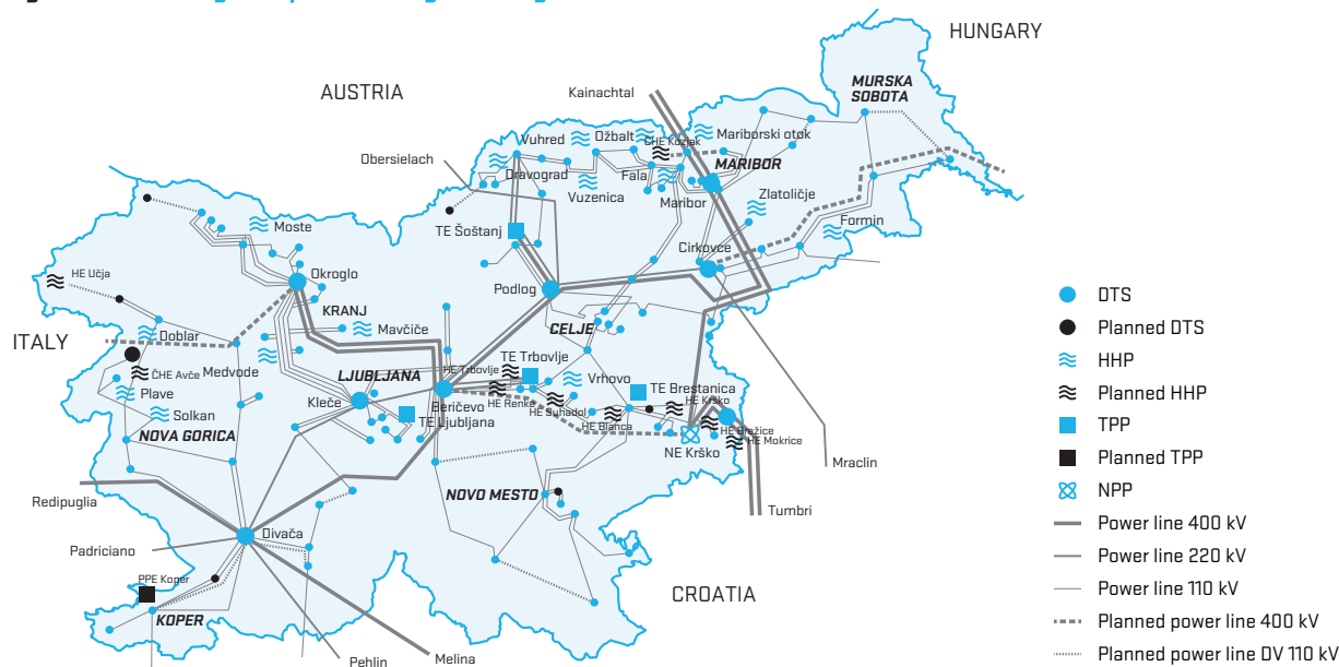
Figure 9: Existing and planned high-voltage network in Slovenia
