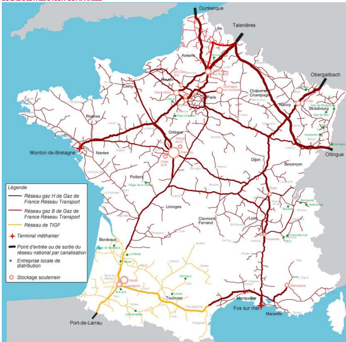
FIGURE NO. 5: NATURAL GAS TRANSMISSION NETWORKS, LNG TERMINALS, UNDERGROUND STORAGE FACILITIES AND LOCAL DISTRIBUTION COMPANIES
