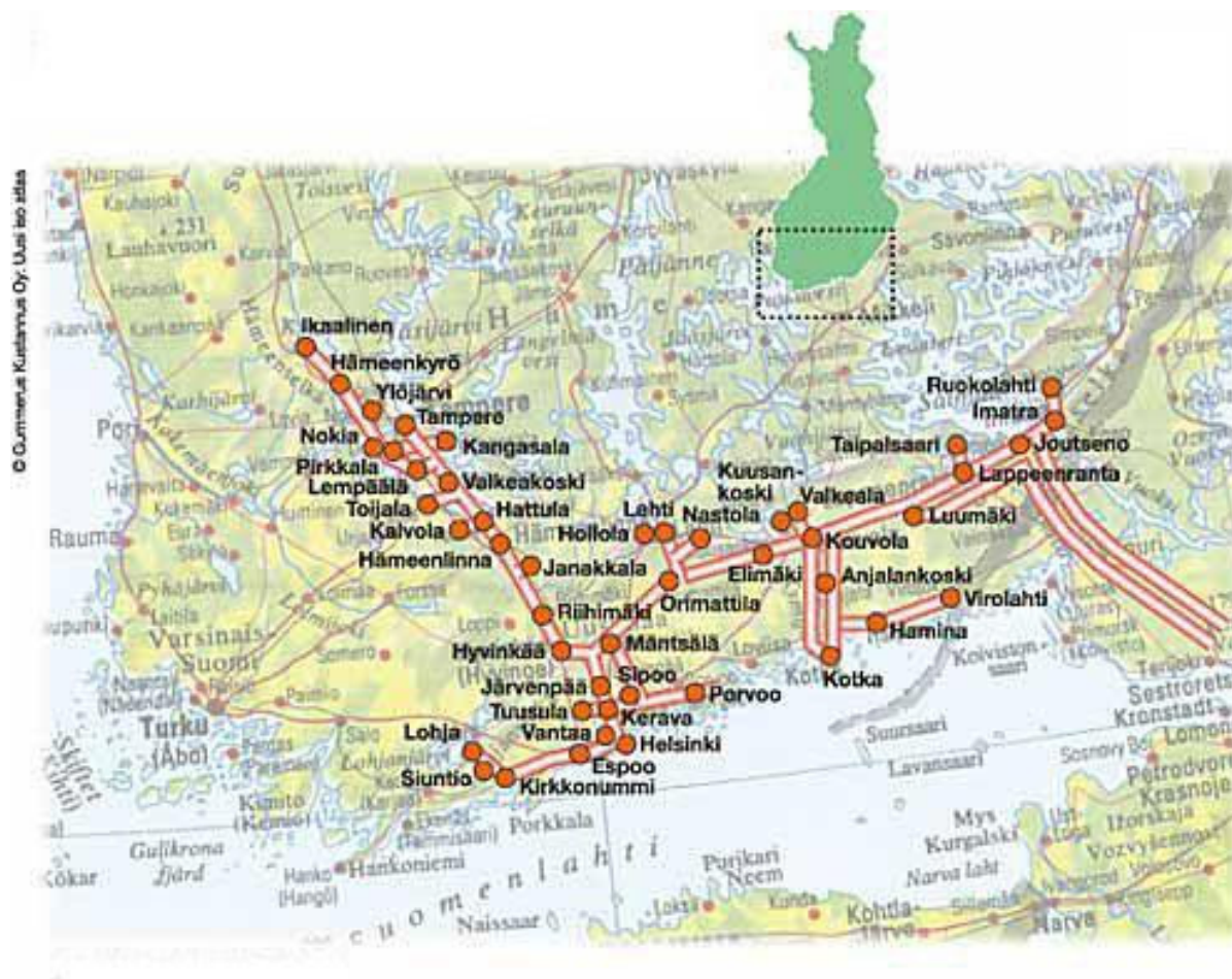
Figure 6. The natural gas transmission network in Finland (Source: Finnish Natural Gas Association)
