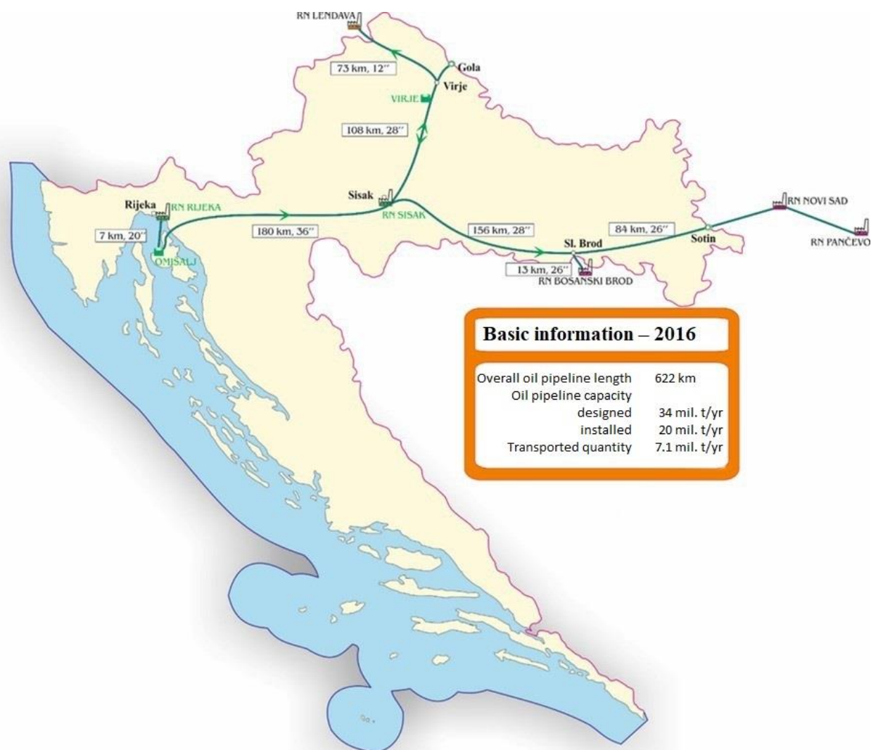
Figure 6.2.1. JANA F d.d. oil pipeline system
