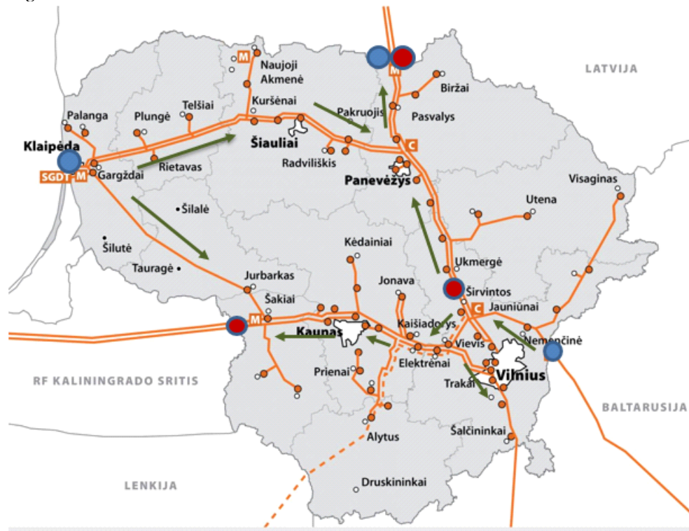
Figure 13. Topological map of the Lithuanian natural gas transmission system according to the Entry-Exit Point Pricing Model
