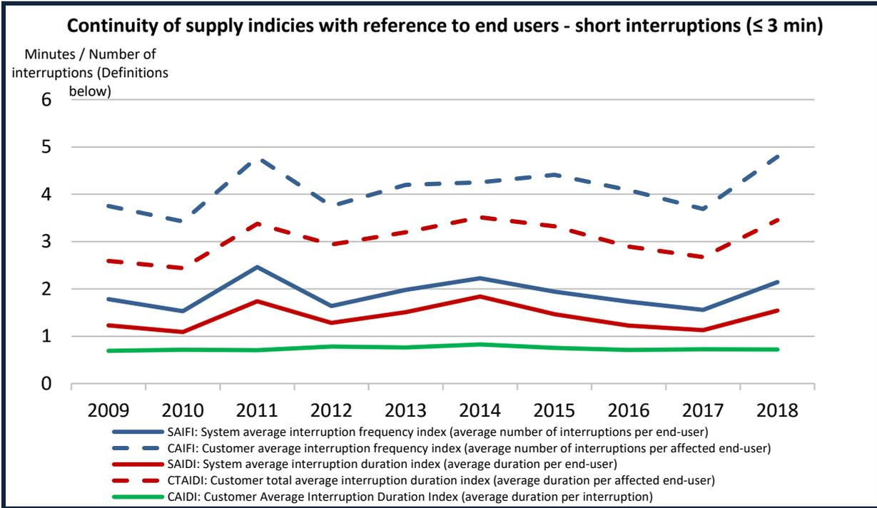
Figure 2. Continuity of supply indices with reference to end users - short interruptions.
