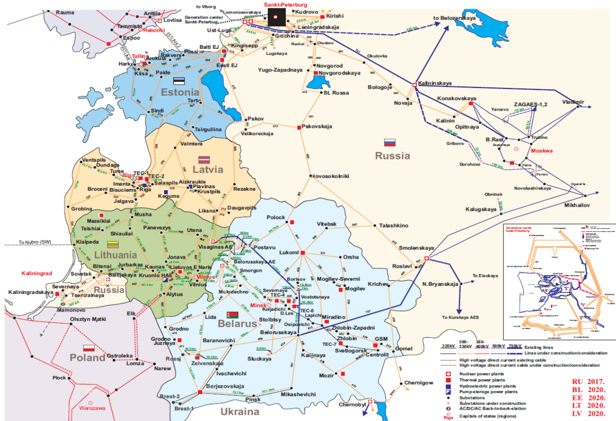
Figure 4. Map of electricity systems of Baltic countries and north-western part of Russia Source: Elering AS
