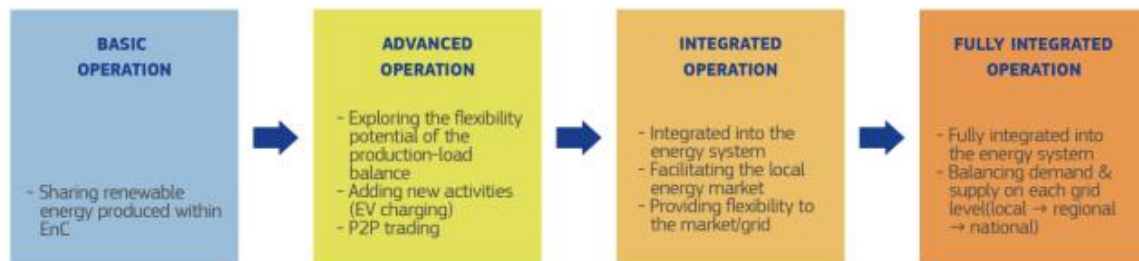
Figure 4-5 Possible transition from basic towards fully integrated operation of energy communities. Source: European Commission (see footnote 76)
