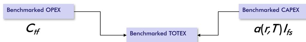
Figure 4-5 Benchmarked Totex = Opex + Capex
